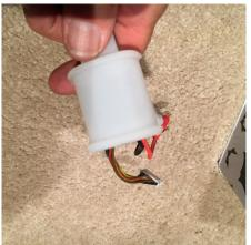
b. Pull wire and wire way seal through opening in box lid as one unit.
